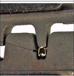
Using the MaxBit stripping Tool (#24140) strip back approximately 1/4 inch (6mm) of casing. See figure #3. We will trim off the excess wire later. Some techs will strip about 1/8 inch and not trim off the rest later.
